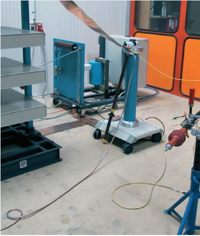
Equipment for impulse test up to 300 kV
