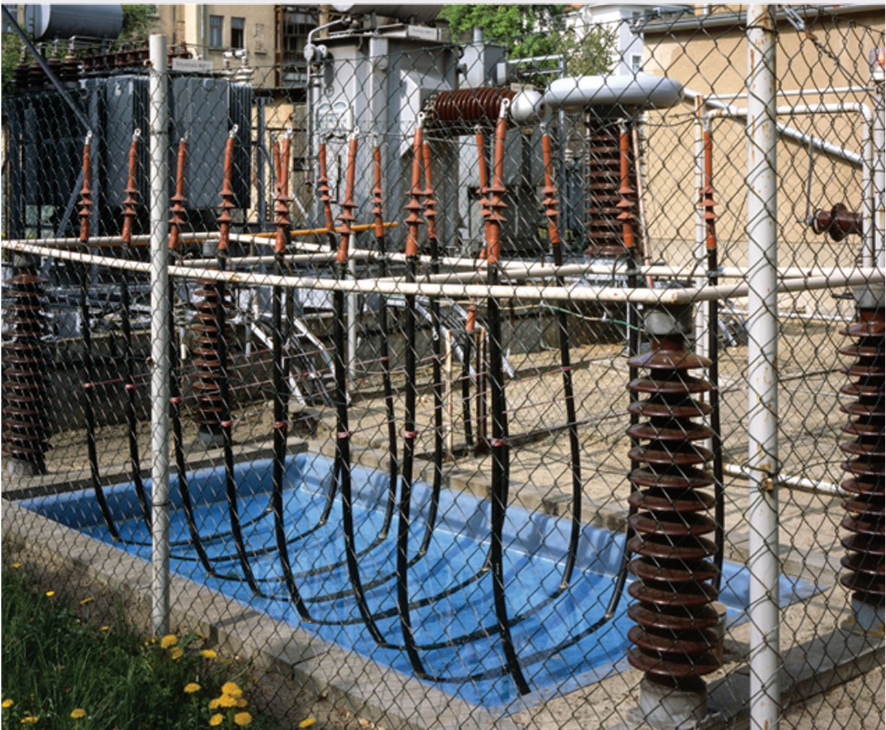
Long term testing of joints and terminations – in air and under water
