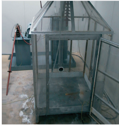
Saltfog chamber with AC transformer 50 kV
