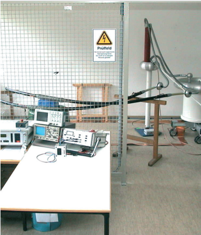
Equipment for partial discharge measurements
