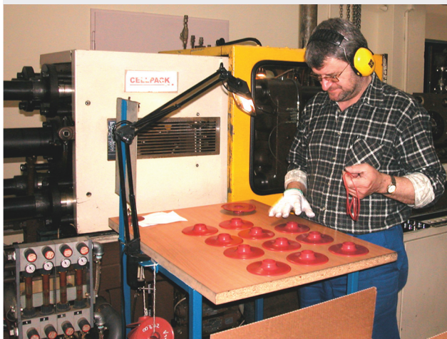
Quality control of silicone sheds ...
